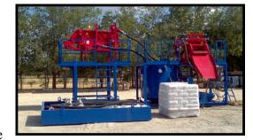
bottom and are transported across our high-speed cuttings shaker screens. The finer solids and **Lubra-Glide Beads** are then pumped to one (1) or two (2) hydro cyclone manifolds mounted atop our high speed cuttings shaker equipped with 150 to 250 mesh screens.
