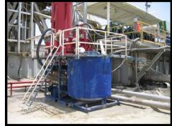
This recovery process allows for 90% - 95% of the Lubra-Glide® Beads to be recovered. This continuous re-introduction of Lubra-Glide® Beads into the drilling and/or completion fluid creates a constant free flowing concentration of beads working downhole to effectively reduce torque and drag conditions.
